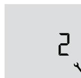
**▶** If the "Service/fault" symbol is illuminated or flashes, you can call up the fault code using the "Menu" button. This menu remains disabled if no fault has arisen.
