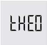
**▶** The tHE0 setting disables the "runtime-dependent rapid heat-up" function. This function is enabled via setting tHE1. The function is disabled at the factory.
