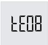
**▶** Set the runtime using the "Plus" and "Minus" buttons. After the set number of hours, the appliance checks whether the set temperature has been reached. If this is not the case, the appliance switches on the electric emergency/booster heater. The factory default is 8 hours.
